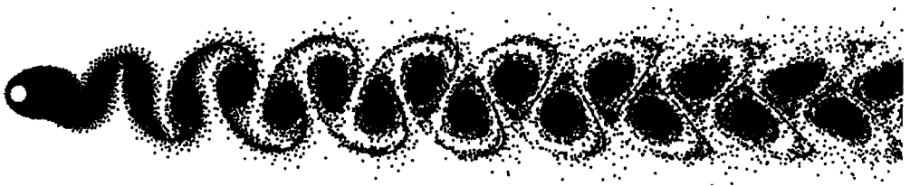
Figure 3. Vortex pattern in the wake, Re = 100 , tU_c/D = 100 .
